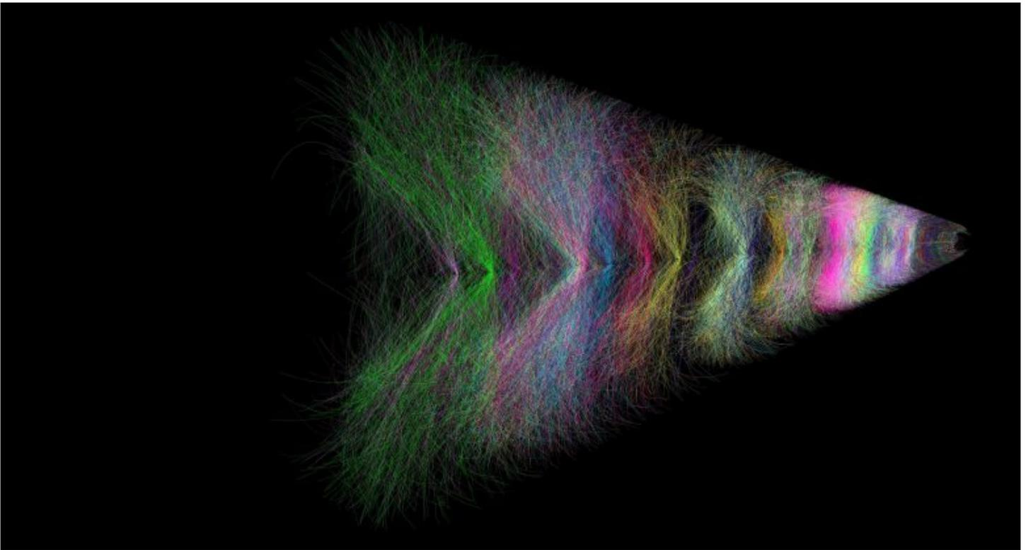
Visualisation of a 2 ms time frame of Pb-Pb collisions at a 50 kHz interaction rate in the ALICE TPC. Tracks from different primary collisions are shown in different colors. Credit: ALICE/CERN
