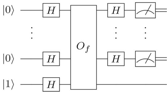
**Fig. 2** Quantum circuit with phase oracle
