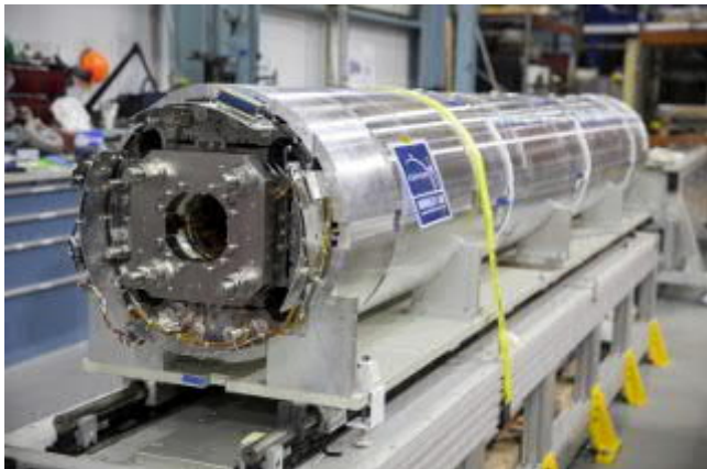
This new magnet -- about as long as a semitruck trailer and weighing 9 tons -- was built by teams at Berkeley Lab, Fermilab, and Brookhaven Lab for the High-Luminosity LHC upgrade project. [Credit: Marilyn Sargent/Berkeley Lab]
